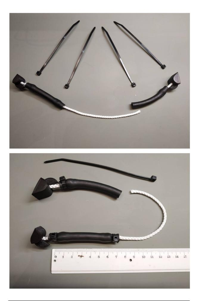
To increase the life expectancy of a string, I recommend using an additional heat shrink tube with a diameter of 4-4.5 mm. Slide the section about 50 mm long over the rope and shrink with hot air.
