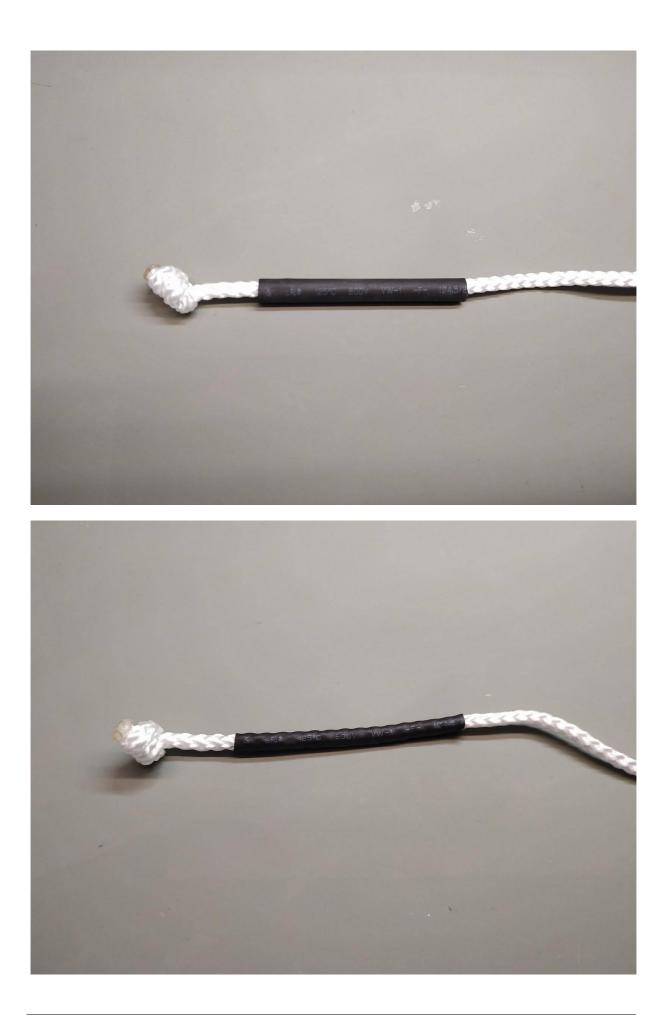
In the last step, we put the middle line through the magazine slot and tie a double loop knot. The knots of the middle part of the rope must be about 10 mm away from *bow\_slider*. Cut the end part of the rope and use lighter.
