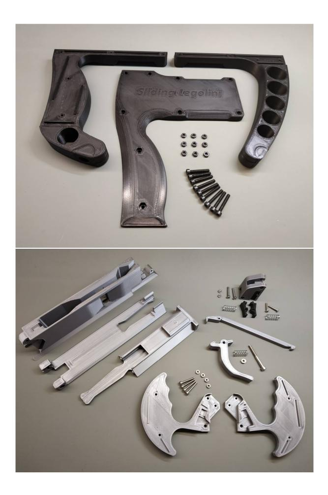
Pay special attention to *bow\_grip* printing. Due to the large rounding of the grip, you need to increase the temperature of the hotend, increase flowrate by 10-15% and reduce the print speed of the shell to 20-30 mm/s on the first 5 layers.
