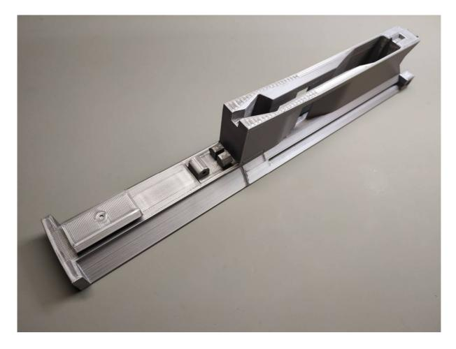
If everything fits, you can split the parts and then glue them together. I recommend using a two-component epoxy adhesive. CA glue is also effective in the case of PLA, but gives a short time for possible adjustments of the arrangement of elements.
